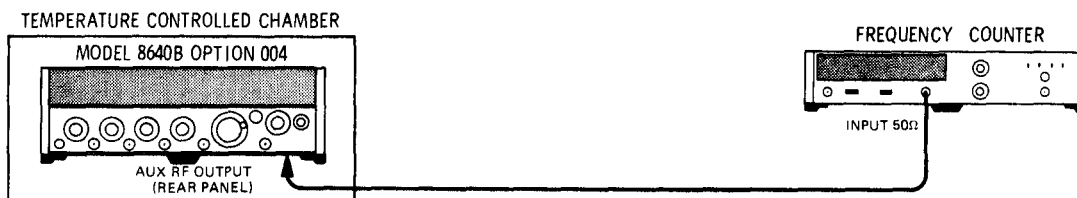
Figure 4-2. Frequency Stability vs Temperature Test Setup
